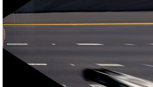
Calibrated video frame number 409 (left) and corresponding overhead view after perspective transform (right).
