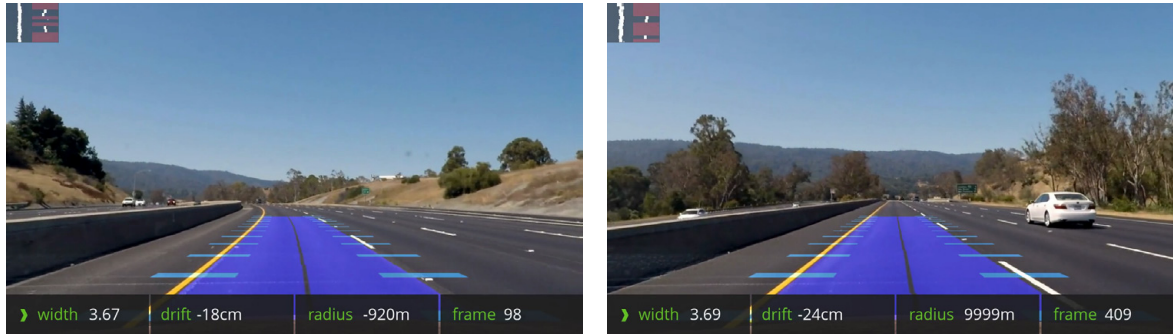
Annotated frames 98 (left) and 409 (right) indicating lane boundaries, curvature, and position from center.
